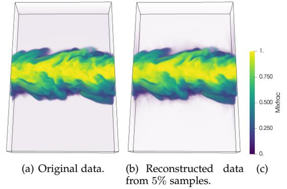
Fig. 7. Volume visualization of Mixfrac field of combustion dataset. Figure 7(a) shows the original data rendering, and Figure 7(b) provides the reconstructed data rendering from 5% sample points. Linear interpolation-based reconstruction is used in this example.
