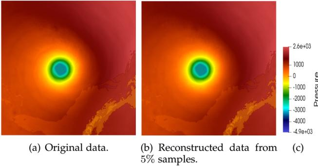
(a) Original data. (b) Reconstructed data from 5% samples. (c) Pressure
