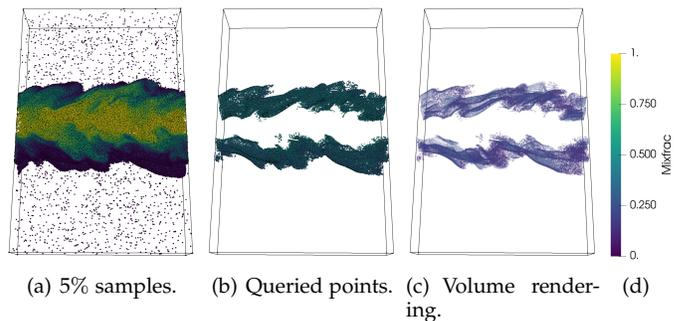
Fig. 6. Sample-based query-driven visualization of combustion dataset on Mixfrac field. Sampling ratio 0.05 is used. Result of an example query of  $\text{Mixfrac} \geq 0.3$  AND  $\leq 0.5$  is shown. Figure 6(a) shows the initial sample points selected. Figure 6(b) shows the points that satisfied the query. Figure 6(c) provides a volume-splat-based visualization of the query results.
