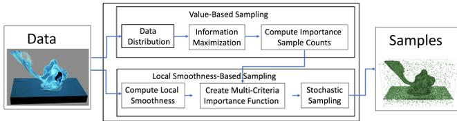
Fig. 1. A schematic workflow diagram of our data-driven sampling approach.
