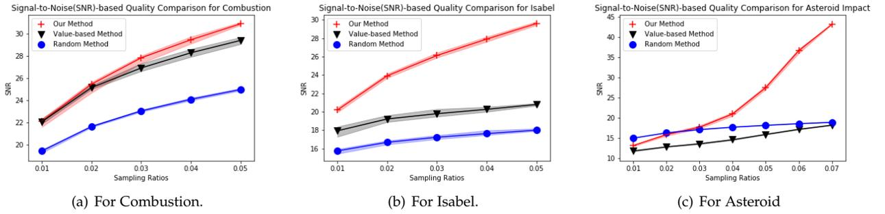
Fig. 16. Comparison of SNR across different sampling methods for three different datasets.
