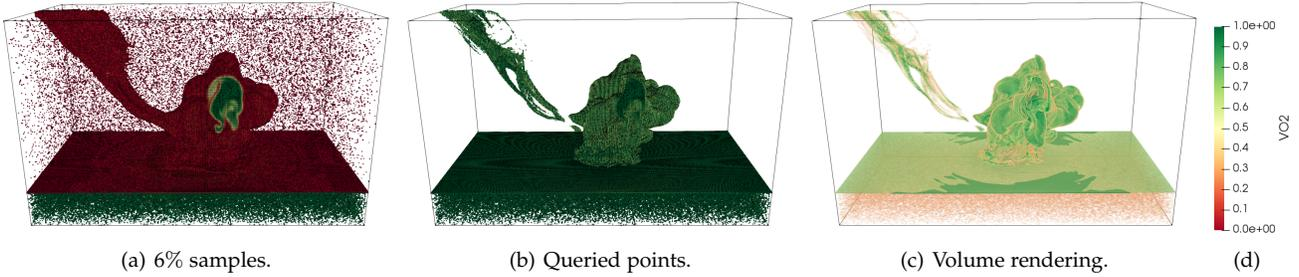
Fig. 12. Sample-based query-driven visualization of asteroid dataset on  $v_{02}$  field. Sampling ratio 0.06 is used. Result of an example query of  $v_{02} \geq 0.75$  is shown. Figure 12(a) shows the initial sample points selected. Figure 12(b) shows the points that satisfied the query. Figure 12(c) provides a volume-splat-based visualization of the query results.
