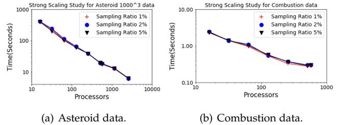
Fig. 20. Strong scaling studies for 1%, 2%, and 5% sampling rates for (a) Asteroid and (b) Combustion data.
