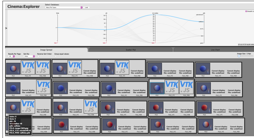
Fig. 9 A simple sphere Cinema database demonstrates the multiple data types in Cinema:Explorer. For each [\phi-\theta] set of parameters, there is an image. Additionally, some of the [\phi-\theta] parameter sets have other data types such as a vtk file or pbd file. Clicking on the thumbnail for each extract (vtk or pbd file) will bring up the data in a viewer for that specific data type, Figure 10.
