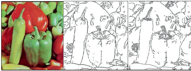
Figure 8. (a) Original pepper image, (b) proposed method output with T=1.2t , (c) openCV canny edge detector (low=70, high=120)
